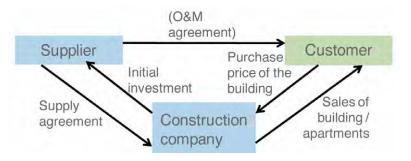
In this model the supplier of the energy system sells the equipment to a construction company. In addition to construction companies these may thus include for example end users or property investors in such cases where these are responsible for the development and planning of the property. In the model the energy system is sold and installed as part of the building project, and sold further to the owner(s) of the building(s). Therefore, the energy system becomes part of the real estate asset.
